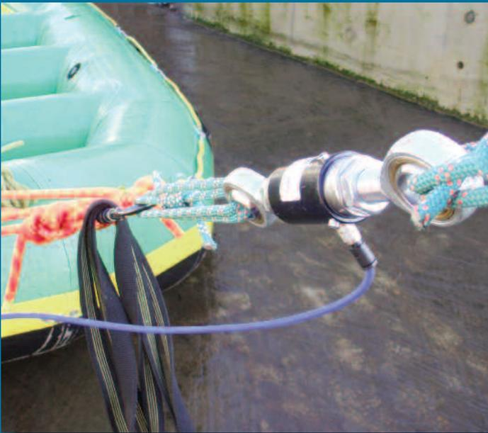
to plane at higher speeds. The value was about 1.3kN but the force became significantly elevated when the crew redistributed themselves at the rear or front of the boat. This redistribution of load influences how the raft is trimmed, and the graph overleaf shows how force changes with respect to trim and water speed. Importantly, the force was relatively constant, or even decreased slightly as the water speed was increased unless the trim was adjusted by moving the crew rear or aftwards.
