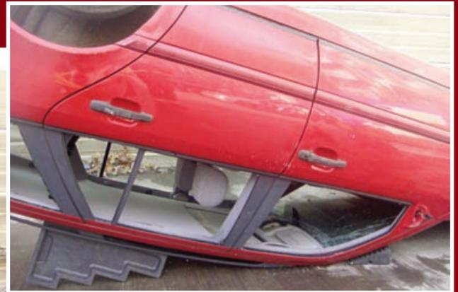
The base of the B pillar can be large and require several cuts if you need to remove the side completely. Alternatively you can take advantage of the space above the vehicle to leave the pillar attached and fold it up and out of the way.
