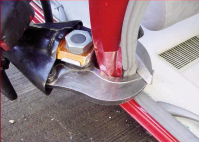
Now cut through the B pillar where it joins the roof
