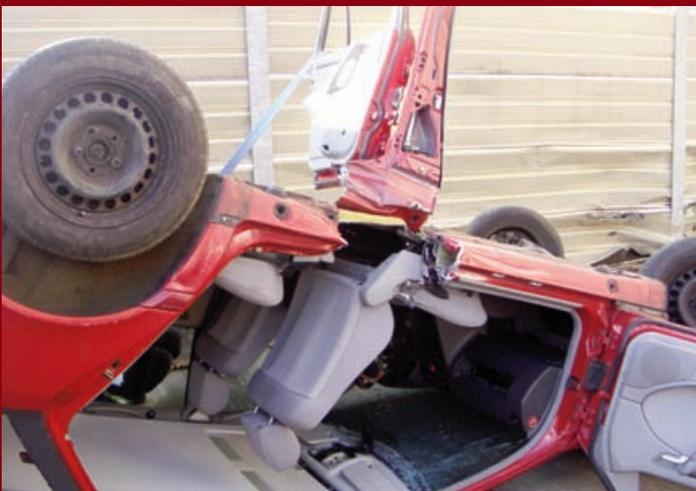
Then fold it up above and out of the way and secure with a ratchet strap
