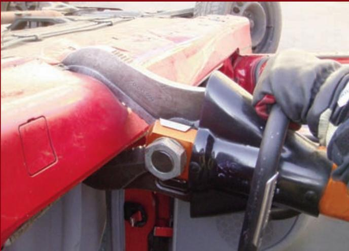
Make a deep relief cut in the sill at 90 degrees immediately behind the B pillar ensuring you cut through the sill completely.
