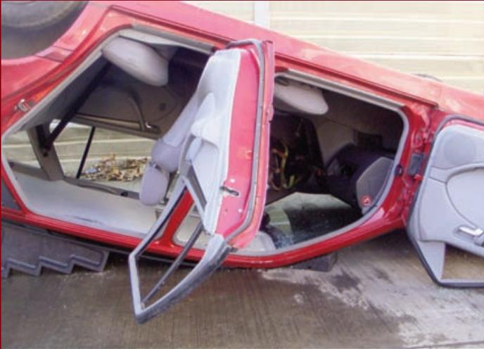
Repeat Steps 1 to 4 to open the rear door. Once this is done, remove all fascia and trim where the 'B' post joins the sill and check for gas generators or associated wiring or tubing. Carry out a risk assessment and implement control measures in accordance with your Brigade, Service or Department protocols and make the following cuts if safe to do so :
